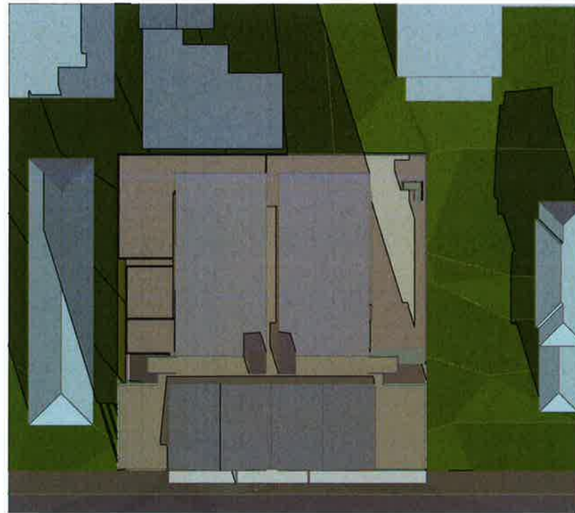
① Shadow Diagram 09am ( Winter Solstice ) Scale 1:400 @ A1 Scale 1:800 @ A3
