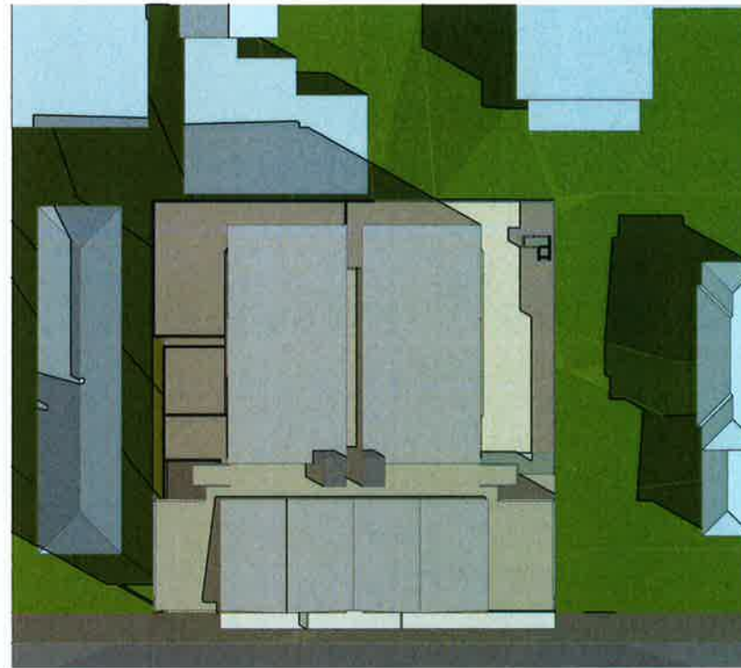
② Shadow Diagram 12pm ( Winter Solstice ) Scale 1:400 @ A1 Scale 1:800 @ A3
